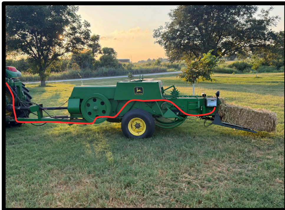
Recommended wire harness path
