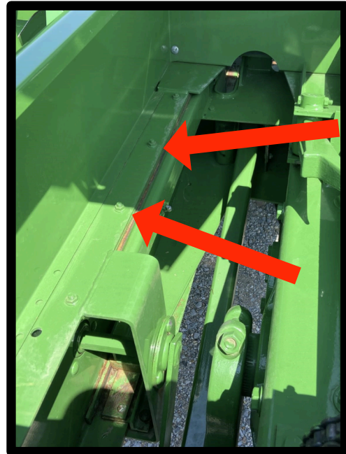
Locate mounting bolts
