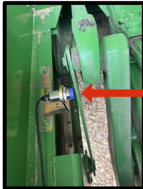
Rotate flywheel so arm is near sensor
