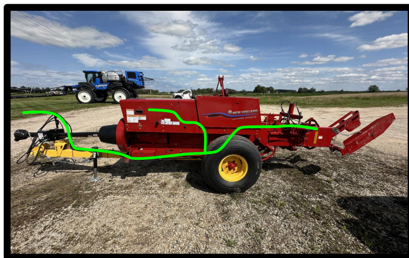
Recommended wire harness path
