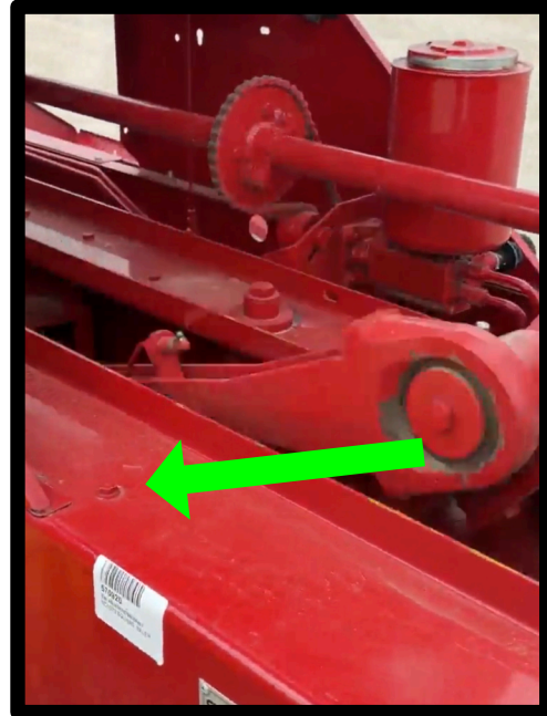
Locate mounting bolt
