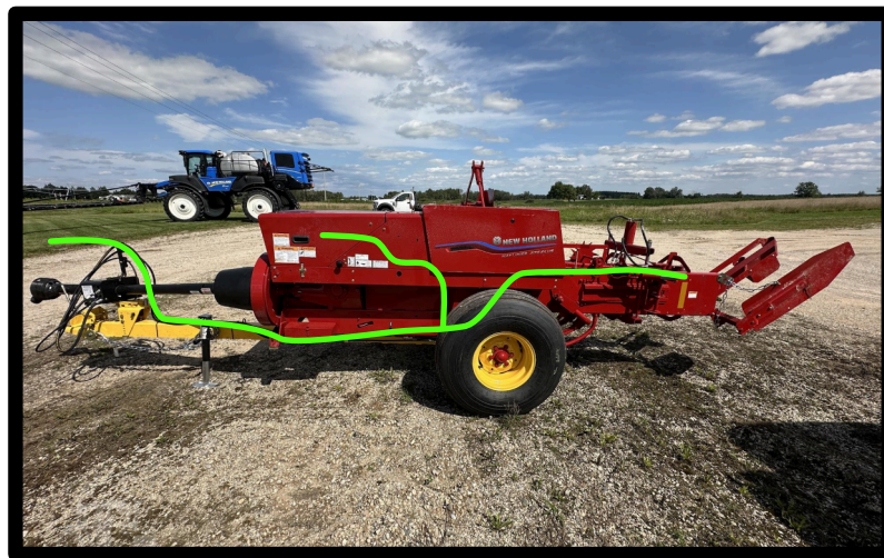
Recommended wire harness path
