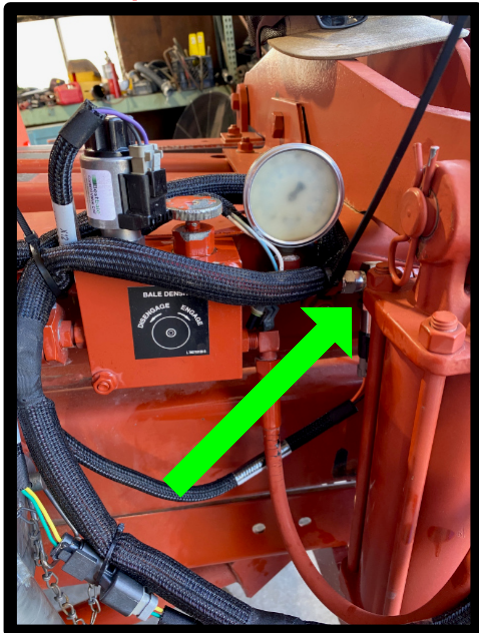
Install with wires down so any moisture drains out of plug
