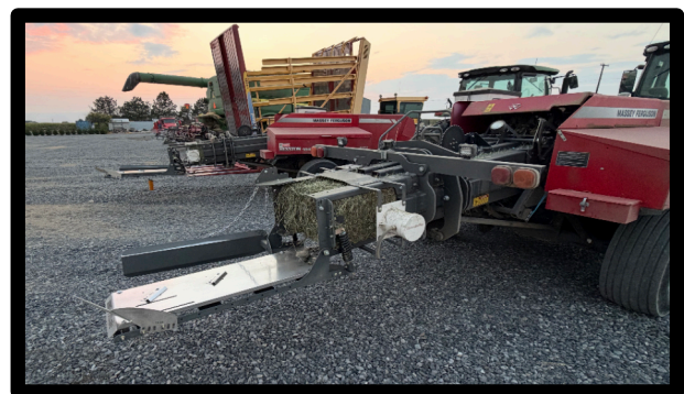
Properly installed ¼ turn scale
