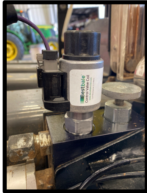
Install BestBale valve & coil Plugs into X12
