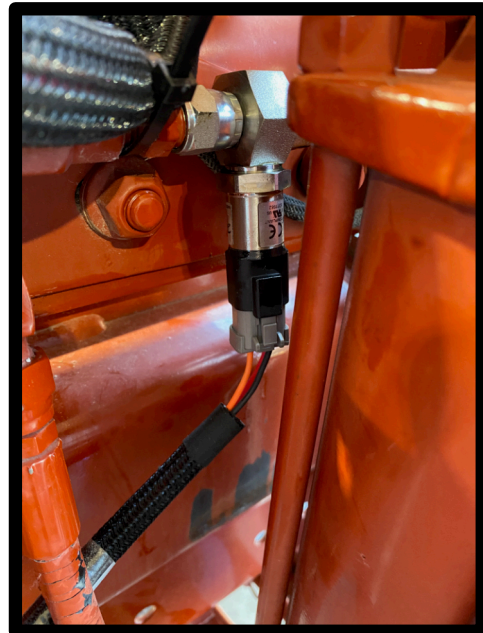
Install with wires down so any moisture drains out of plug
